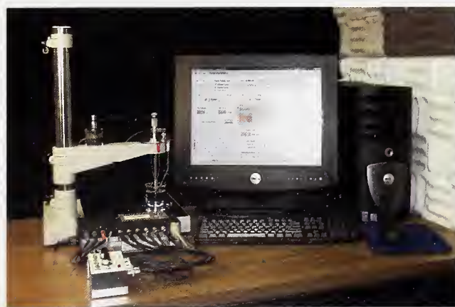
Figure 2. Fully automatic computerized nano-tip fabrication apparatus.
